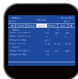
UPS Cabinet Control Panel
