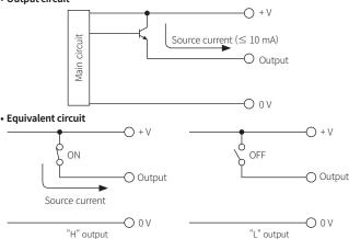
Connection example of PNP open collector output type and external application circuit
