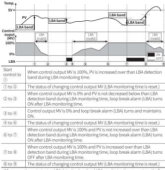
When executing auto-tuning, LBA detection band and LBA monitoring time are automatically set based on auto tuning value. When alarm operation mode is set as loop break alarm (LBA), LBA detection band and LBA monitoring time parameter is displayed.
